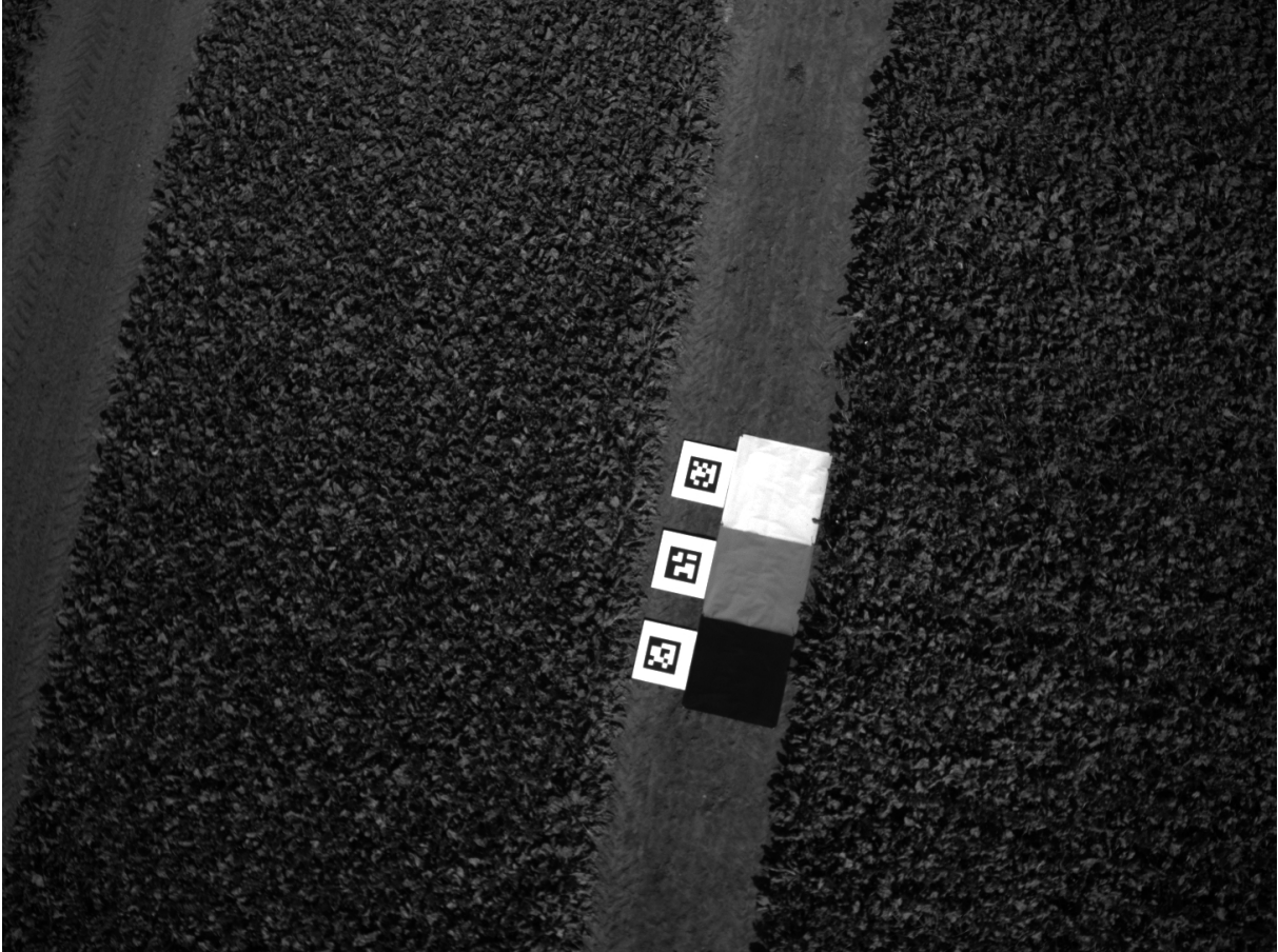
Figure 4: 3 AprilTags of the tag25h9 family placed next to 3 calibration targets
